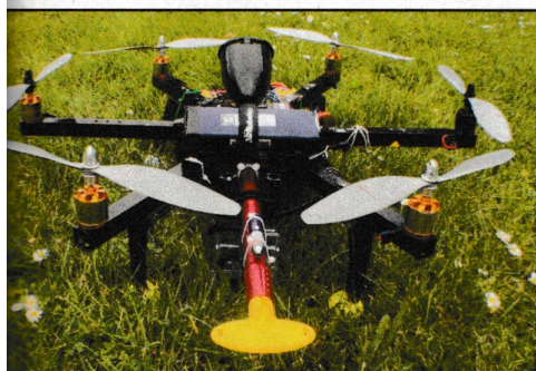
Nowhere to hide: a heavy-lift drone, mounted with a high-capacity automatic paintball gun. 📺 AERIAL SPORTS LEAGUE
